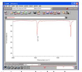
When comparing spectra, overlay works better in color and stacked works better in black and white. You can switch between them using the toggle icon.
