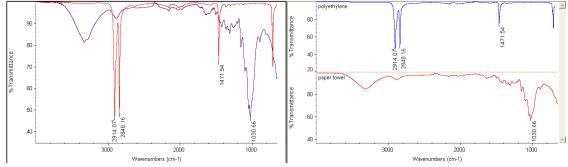
You can search for a spectral match in a library. (If some peaks are offscale you can select only a portion of the spectrum for matching by clicking on the Select a Region tool and dragging on the spectrum.) Click on the Search for Spectral Match icon for a list of possible compound identifications. To create a new library use menu Analyze/Library Manager/Create Library with type equal to search. To add spectra to a library click on the Add to Library icon.
