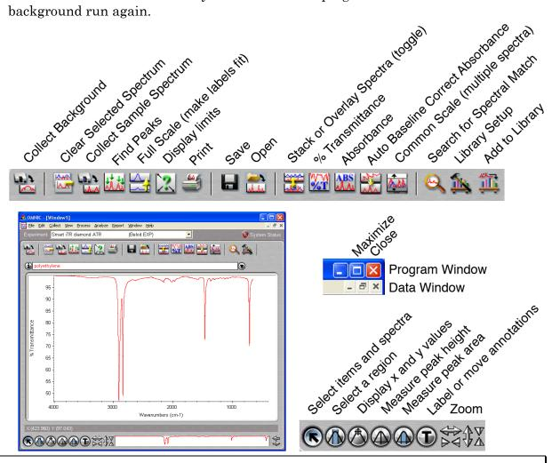
Put the sample in the instrument. For solid ATR turn the knob just until you hear a click. Click on the *Collect Sample Spectrum* icon. Title is part of the printed report. The spectrum will be displayed after collection. Add to window: Yes.
